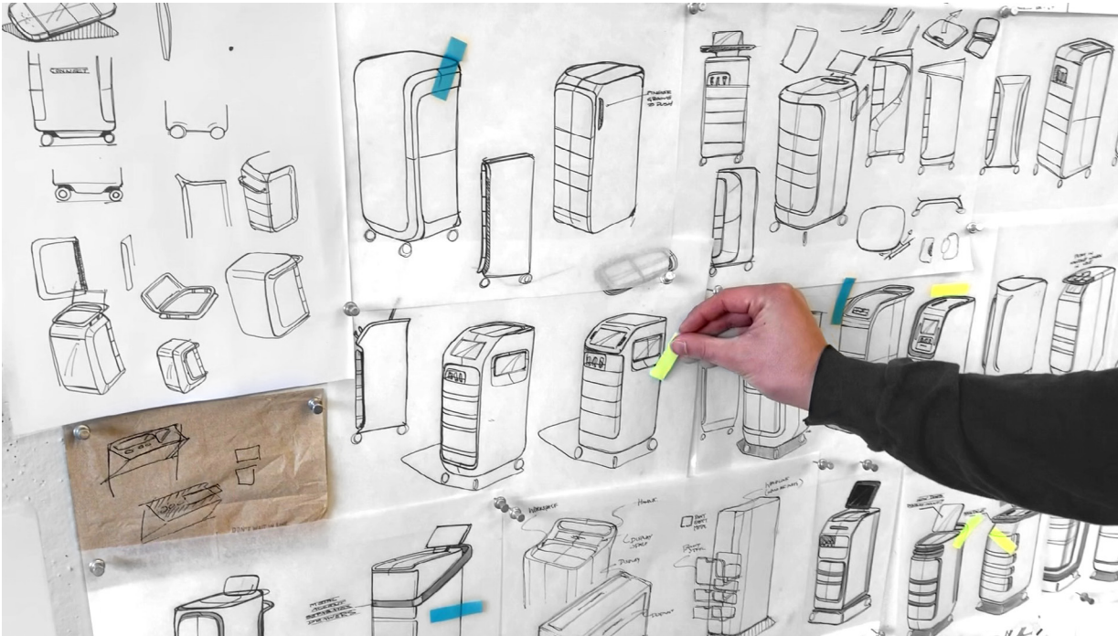
The rough sketch phase involved sketching over the different internal layout concepts. Focusing on the first read, this phase explored a variety of forms and proportions. Using blue tags for overall form and yellow for details, an internal ID review with classmates helped down select ideas heading into the refined sketch phase.
