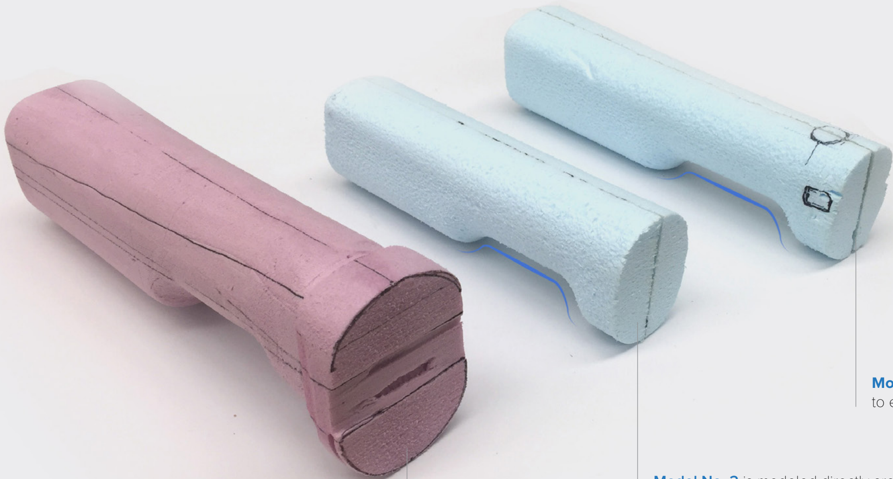
Model No. 2 is modeled directly around the internal components resulting in a slimmer, more ergonomic design .
